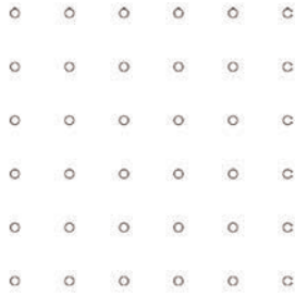
Hole size: Dia 0.8mm Pitch: 5.0mm Open Area: 2.0%
